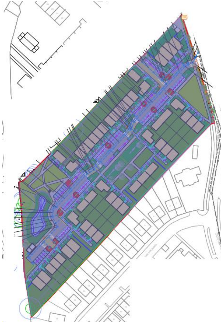
Figure 2.1 – Surface Water Drainage Catchment Area
