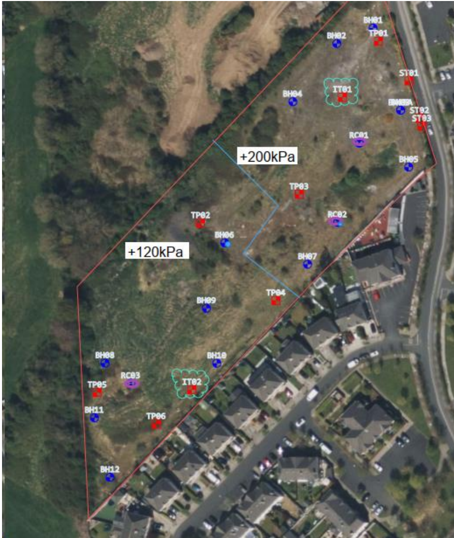
Figure 2.9– Site plan for site investigation works (Source: Causeway Geotech site investigation report No. 23-0881E)
